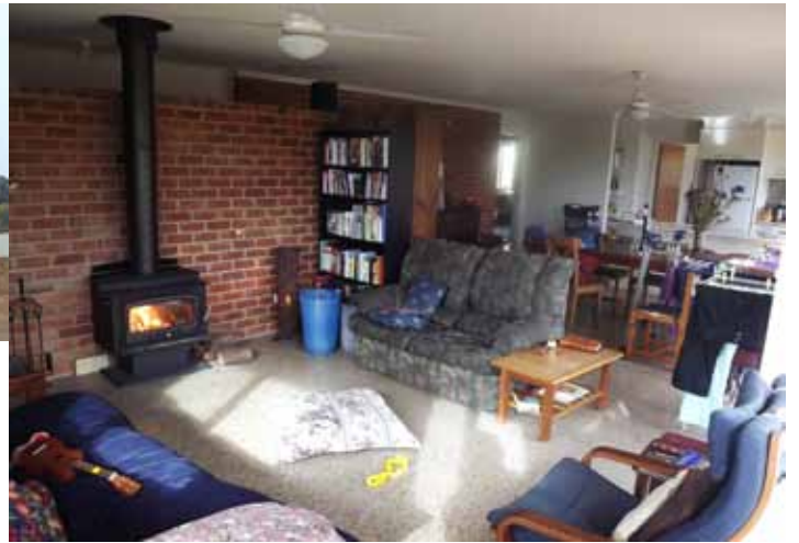
Manna Gum's new home (cont.): passive solar design is a simple concept that combines using a northward orientation, internal thermal mass, eaves, double glazing and heavy insulation to provide warmth in winter and coolness in summer; (above) view from the street - the house opens to the north to capture the winter sun; (right) living space - heats by sunlight when the sun is out and wood heater when it is not.
