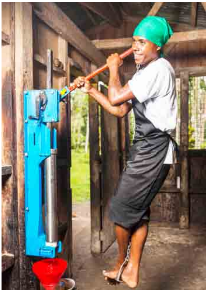
Left: The Direct Micro Expelling technique provides a cheap and easy-to-use means of village-based production of high-value coconut oil. Below: a four-man team at the drying tables. Photos by Sean Davey.
