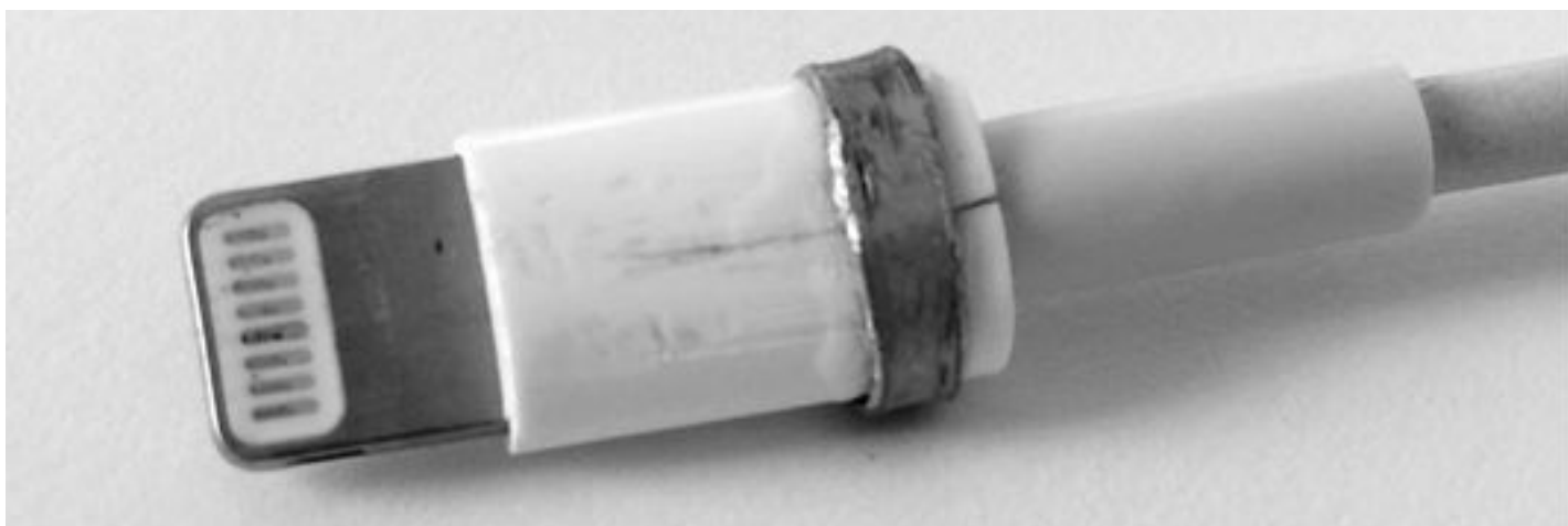
A metal ring ensures this high-use item stays functional as long as possible after mending.
