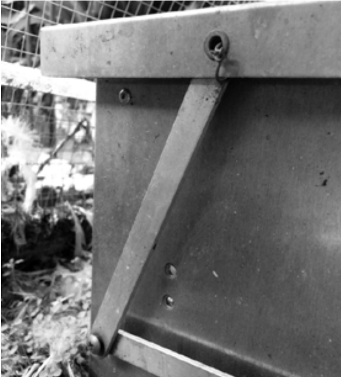
A twist of wire replaces a problem bolt on this chicken feeder.
